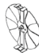
Detail (A) (Radial sliding blade damper)
